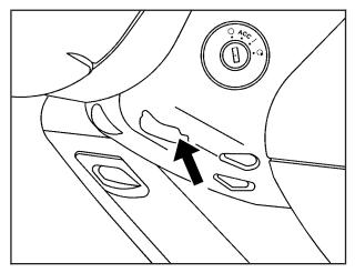
2. Using a tool, pry off the cover from the bottom of the steering column.
